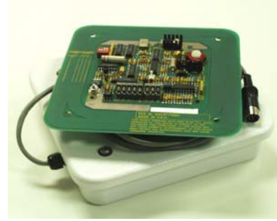
Model 1885E Combo Multiplex Reader/Read Head FCC Approved Addressable Approximate size is 8" x 8" x 1.5"
