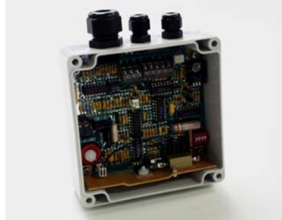
Model 1845E Multiplexing Reader FCC Approved Addressable Approximate size is 4.75" x 4.75" x 2"
